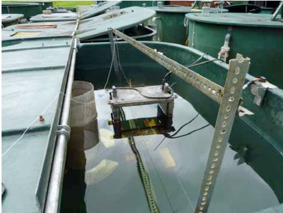
Figure 1: Vaki Riverwatcher fish counter experimental arrangement.
