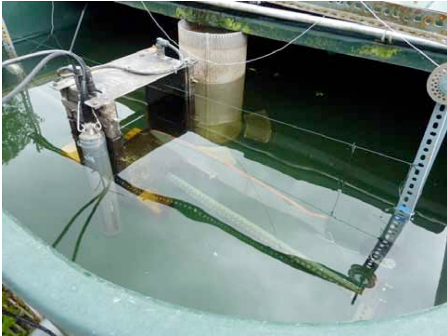
Figure 3: Vaki Riverwatcher counter, turbidity probe and fish target under clear conditions (0 NTU).
